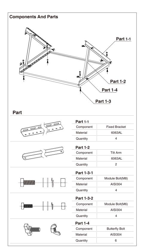
Assemble the components and parts together according to the left picture. Attached the PV module to the mounting brackets using M8 screw/bolt supplied in the pack. Be carful of the bolt, flat washer, spring wash and nut sequences. Find suitable holes on the panel frame and tighten the brackets on it.
